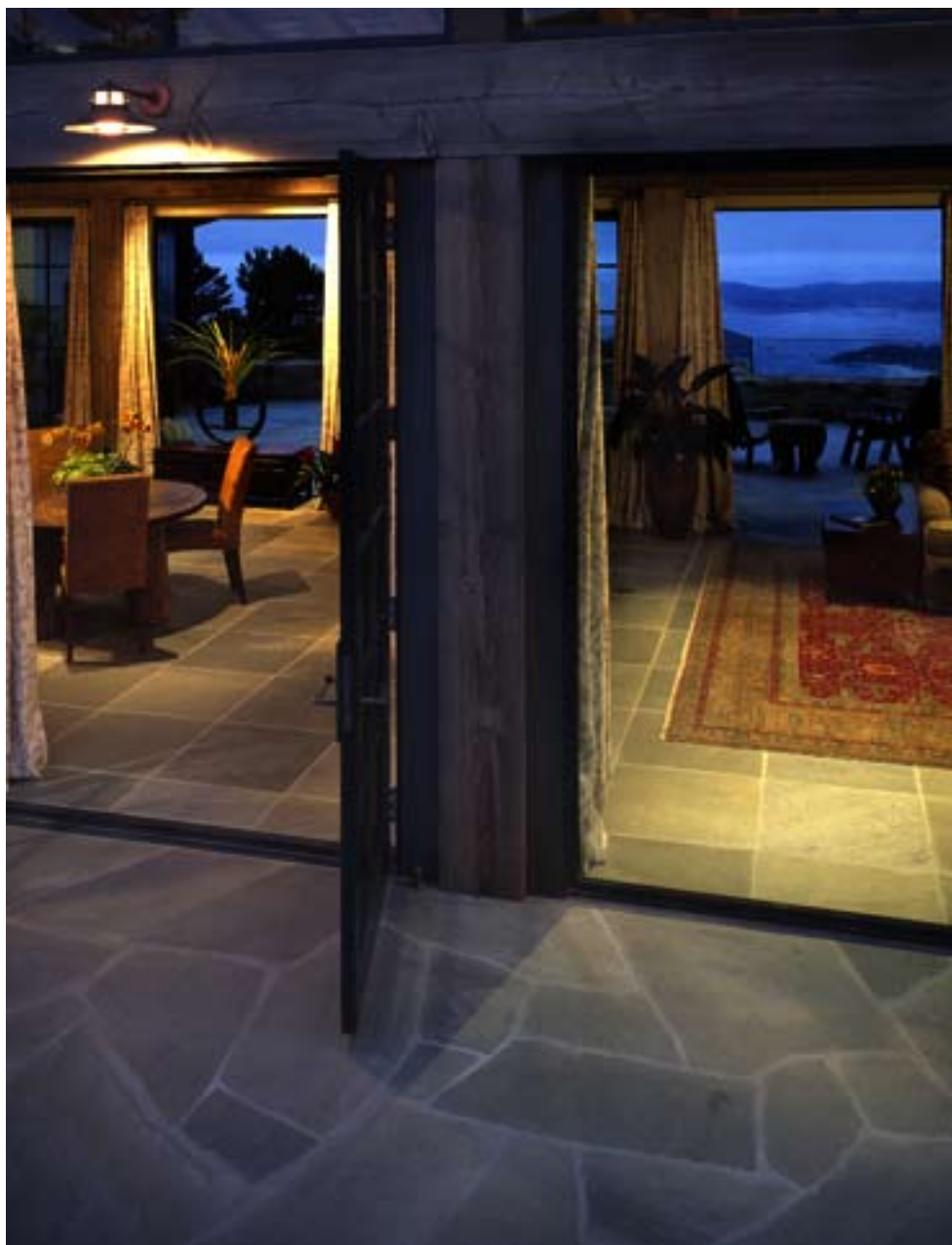
To take better advantage of the sun, the home's owners cut into the uphill slope and created a courtyard behind the house (left). They also used lots of glass (above), allowing light to flood the interior, where it warms the stone floors, which also serves to heat the interior at night (below).
